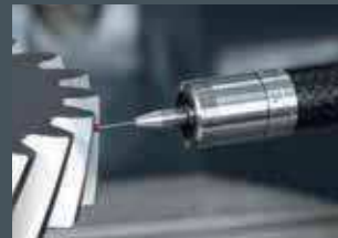
Workpiece measurement in grinding centre
