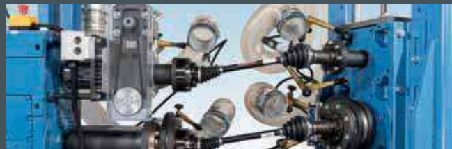
Drive Shaft Test Stands
