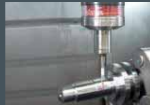
TC63-30 – application in turning-milling centre
