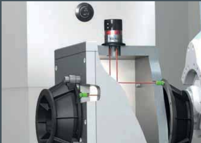
Integration of sensors (temperature, workpiece position, clamping pressure) in the workpiece clamping device. Wireless data transmission via BRC-Technology.
