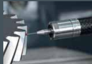
Workpiece measurement in grinding centre
